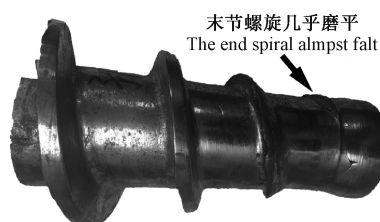
图 2 失效的膨化螺杆挤压输送段 Fig.2 Failed extrusion conveying section
