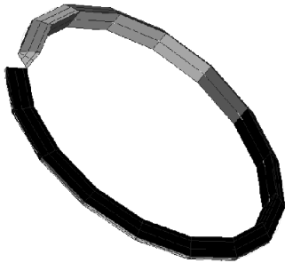
(b) 外螺纹一个螺距内的三维网格 (b) 3D element of external thread in one pitch
