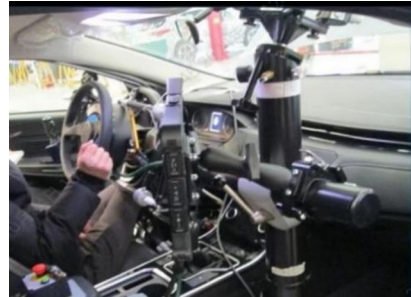
图 15 测力转向盘与V-BOX测量系统 Fig. 15 Force measuring steering wheel and V-BOX measurement system
